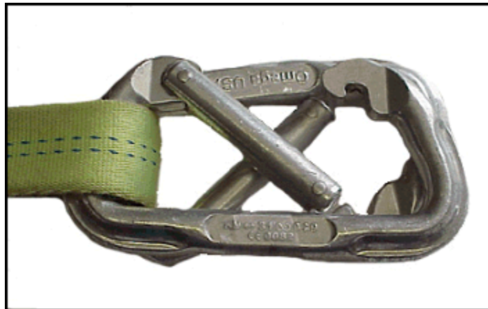
Figure 5-6. Correctly opposed carabiners.
