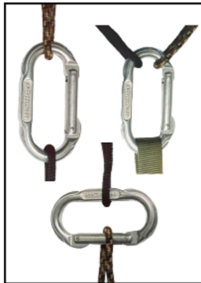
Figure 3-12. Major and minor axes and three-way loading.
